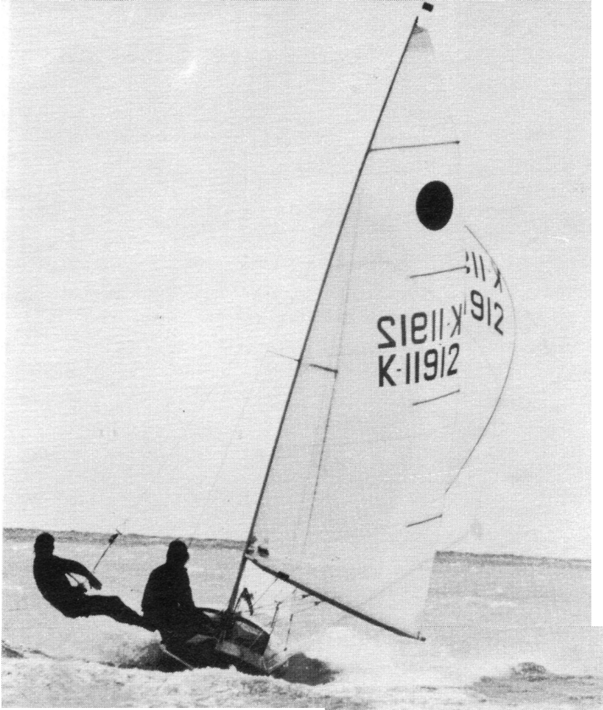
Smith again, sitting on the edge of his scat on a windy three-sail rcach. Note: kicker well off; main well out.
